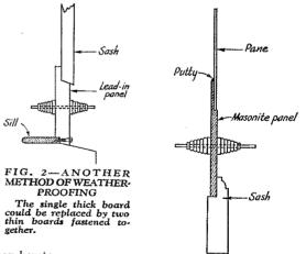
FIG. 3—A METHOD WHICH AVOIDS DRILLING HOLES IN GLASS
