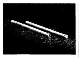
SPREADER: Light in weight as well as exceptionally efficient, these NATIONAL spreaders offer unusual advantages. The material is non-hydroscopic and weatherproof. The slender shape minimizes surface leakage. The power factor is of the order of 0.15%. The weight is but one ounce each. Catalog Symbol AA-3.
