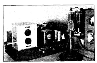
THE PENTODE INPUT STAGE ELIMINATED R.F. PICKUP IN THIS SPEECH AMPLIFIER UNIT BUILT BY THE AUTHOR FOR THE BOWDOIN EXPEDITION STATION, VEIIN
