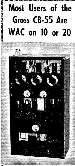
The CB-55 RADIOTELEPHONE and telegraph transmitter offers the user one of the finest units of its kind at an unheard of price, employing the latest circuits and beautiful workmanship. The use of the new T-20's in the output stage assures the user the possession of a commercial looking installation of a real power output and broadcast station quality.
