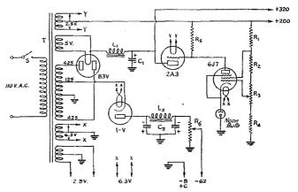
FIG. 3—REVISED POWER SUPPLY DIAGRAM, WITH BIAS SUPPLY INCLUDED
