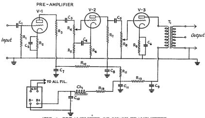
(FIG. 1—PRE-AMPLIFIER OF OX2QY TRANSMITTER -8000-ohm, 1-watt (IRC).  $R_2-$ Rs-250,000-ohm v.c.,
