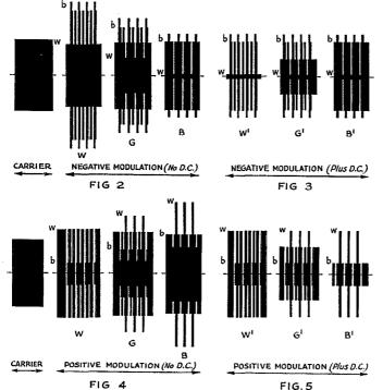
FIGS. 2, 3, 4 AND 5-FOUR TYPES OF TELEVISION SIGNAL R.F. WAVES REPRESENTING SCANNING OF SIMPLE IMAGES
