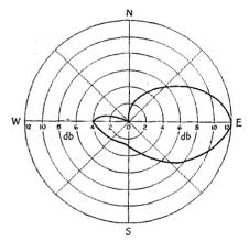
FIG. 2-RADIATION PATTERN PLOTTED IN DB ABOVE MINIMUM FIELD STRENGTH IN N.W. DIRECTION
