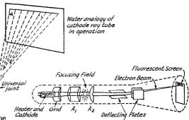
FIG. 1—ILLUSTRATING THE PICTURE-REPRODUCING ACTION OF THE CATHODE-RAY TUBE
